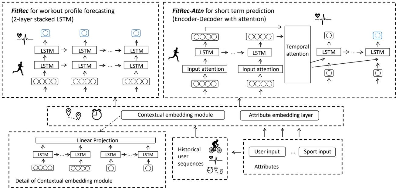
**Figure 3: Model structure for workout profile forecasting (*FitRec*) and short term prediction (*FitRec-Attn*). *FitRec* contains a 2-layer stacked LSTM and *FitRec-Attn* has an encoder-decoder module with dual-stage attention. The final outputs are colored in blue.**
